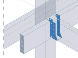
DETALLE 3: Unión Pilar - Piso
