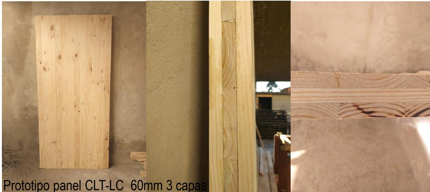
Prototipo panel CLT-LC 60mm 3 capas
