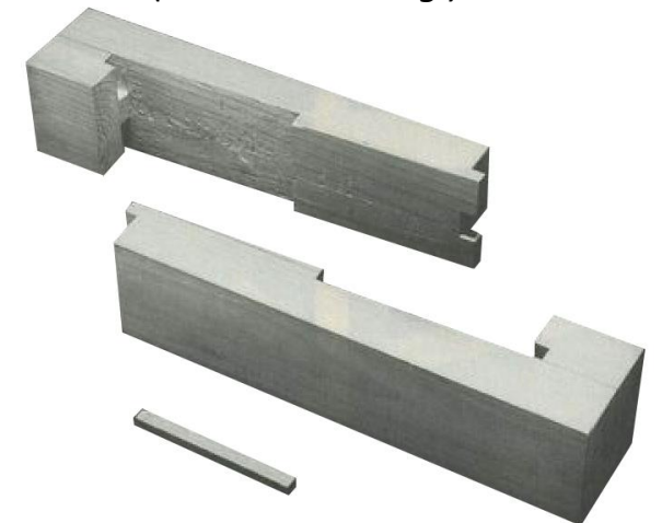
Blind stubbed, housed rabbeted oblique scarf splice (Shiribasami tsugi)
